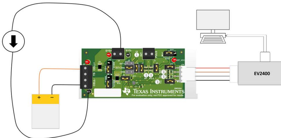
**Figure 2-8. Current Calibration Hardware Setup**
