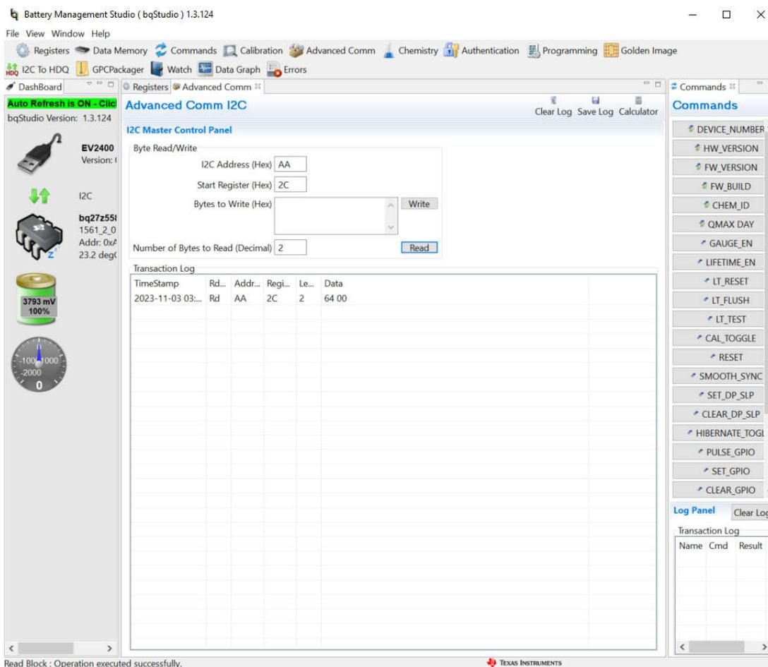
Figure 3-3. Standard Data Command Example
