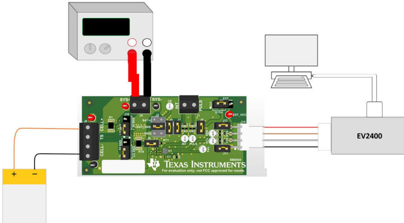
Figure 2-1. Connect the BQ27Z558 Circuit Module to a 1SxP
