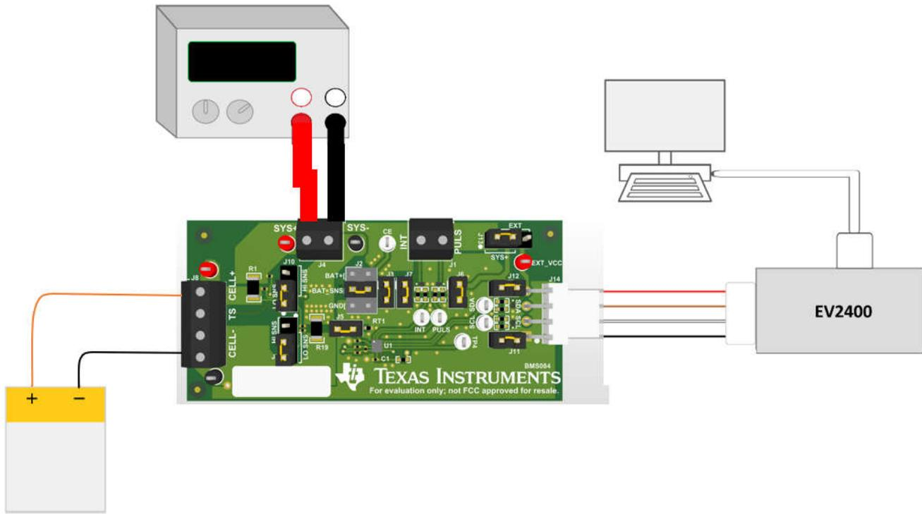
**Figure 2-3. ChemID Hardware Setup**
