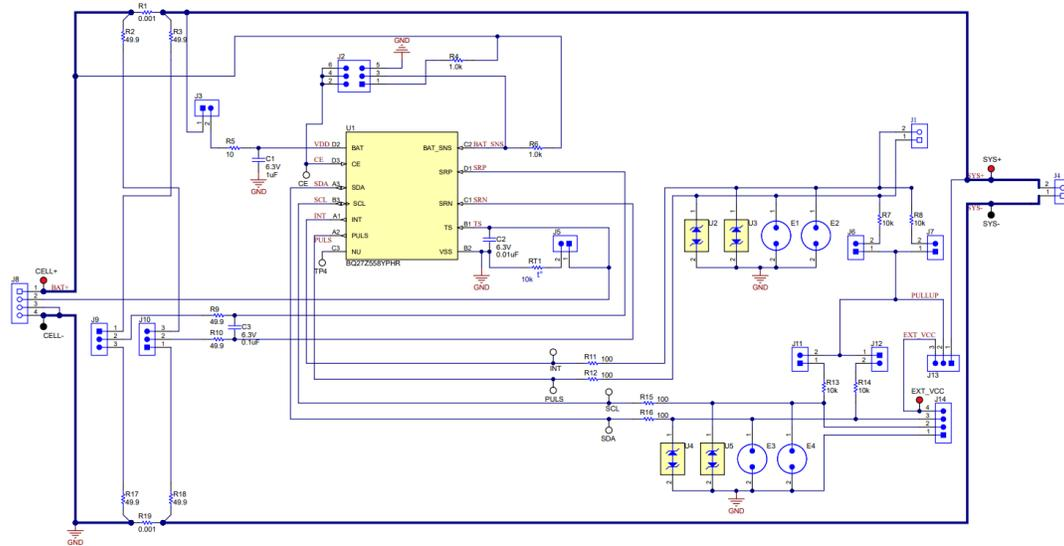
Figure 4-1. BQ27Z558 Reference Schematic
