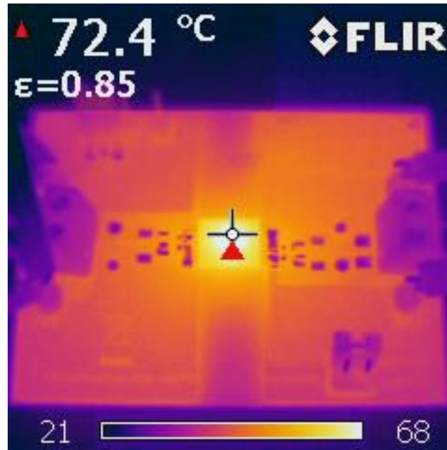
Figure 3-24. UCC33421-Q1 VINP=5.0V, VCC=5.0V, I out =300mA, P out =1.5W, TA=25°C
