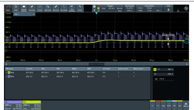
Figure 3-48. 1KV Surge at 230Vac input
