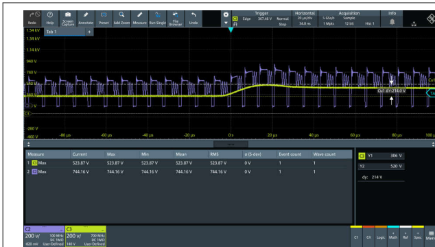
Figure 3-47. 2KV Surge at 230Vac input
