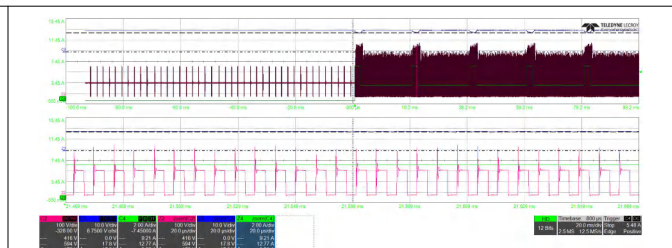
Figure 3-52. VIN=90Vac (2x rated current for 2ms, 0.9x rated current for 18ms) - Zoomed
