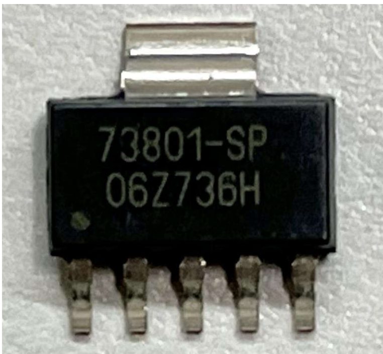
Figure 1-1. TPS73801-SEP Device Photo
