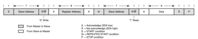
Figure 8-7. "Read" Data Transfer Format in Standard-, Fast, and Fast-Plus Modes
