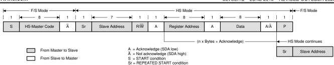
Figure 8-8. Data Transfer Format in HS-Mode
