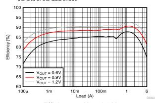
Efficiency at V<sub>IN</sub> = 3.3 V
