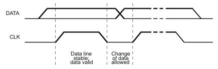
Figure 8-3. Bit Transfer on the Serial Interface
