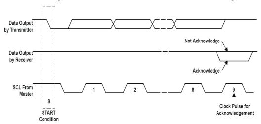
Figure 8-4. Acknowledge on the I<sup>2</sup>C Bus
