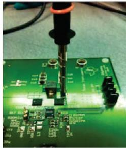
**Figure 10. Testing Switch Node**
