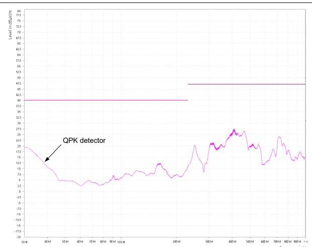
Figure 5-30. CISPR 32 Class B Radiated Emissions: Vertical Polarization
