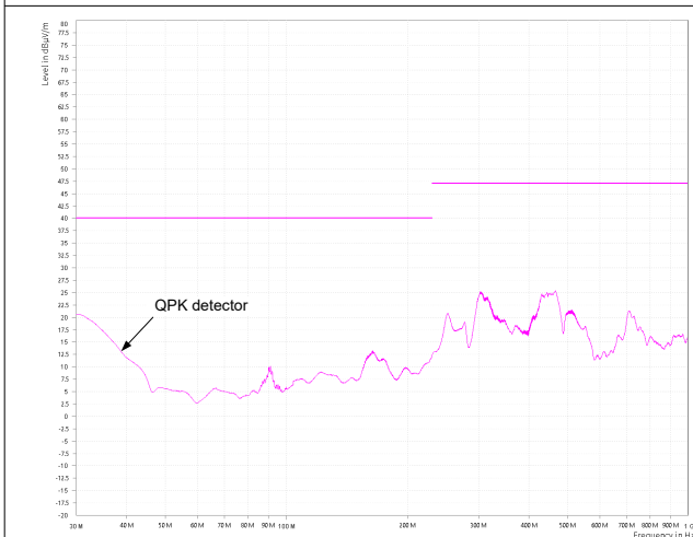
Figure 5-29. CISPR 32 Class B Radiated Emissions: Horizontal Polarization
