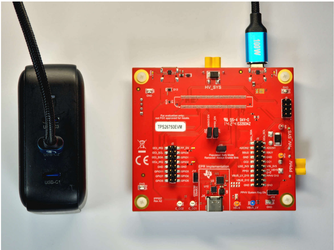
Figure 2-4. Stand Alone Testing Example Hardware Setup
