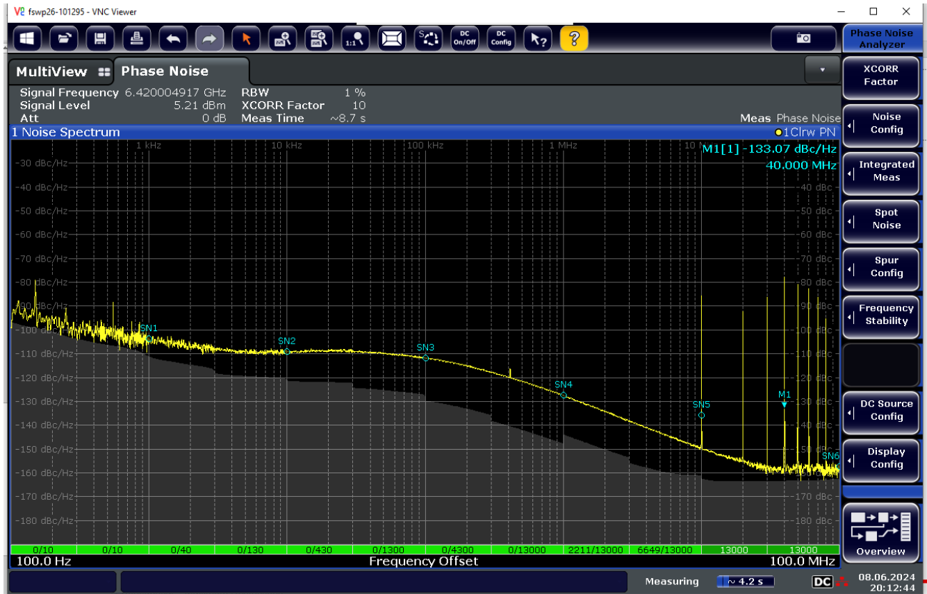
Figure 16. Third Order (Silicon PN Plot) With Charge Pump Gain Reduced
