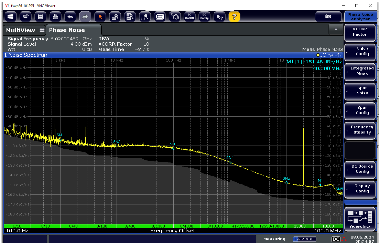
Figure 22. Third Order MASH (Silicon PN Plot) With Charge Pump Gain Reduced and Slight Change in Fraction
