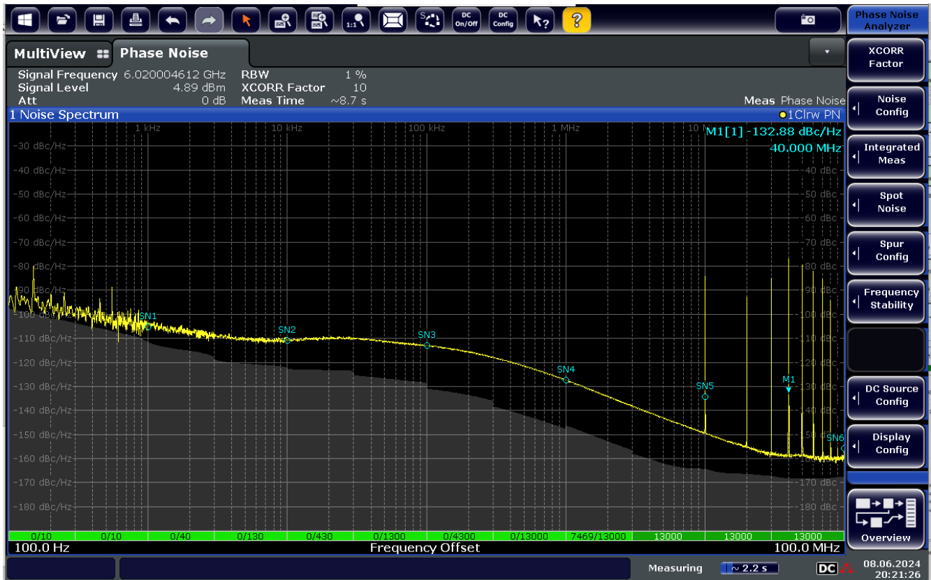
Figure 21. Third Order MASH (Silicon PN Plot) With Charge Pump Gain Reduced
