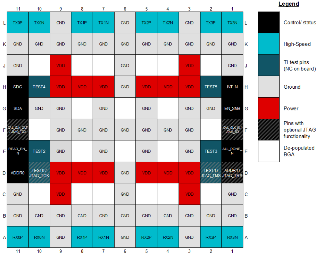
Figure 2-2. DS250DF410 Pin Configuration
