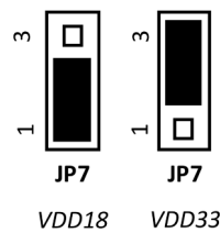
Figure 3-2. VDDIO Select (JP7) Jumper Settings
