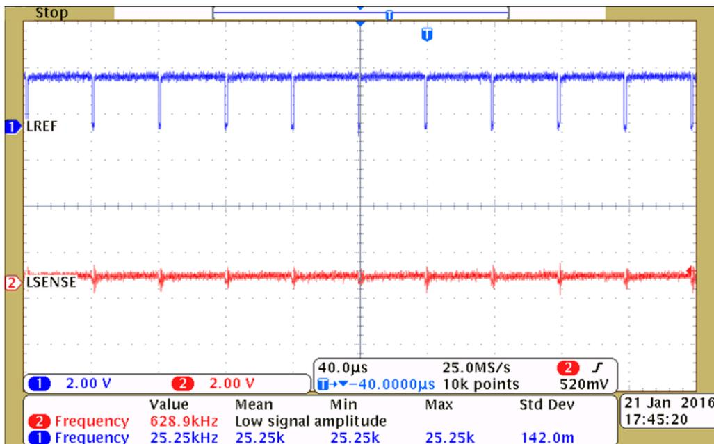
Figure 3. LREF Disconnected
