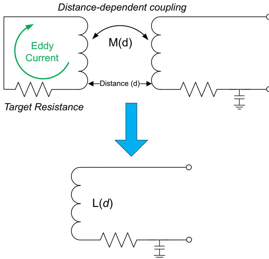
**Figure 1. Series LC Configuration in the LDC0851**
