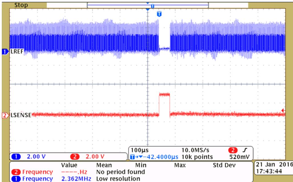
Figure 2. LSENSE Disconnected
