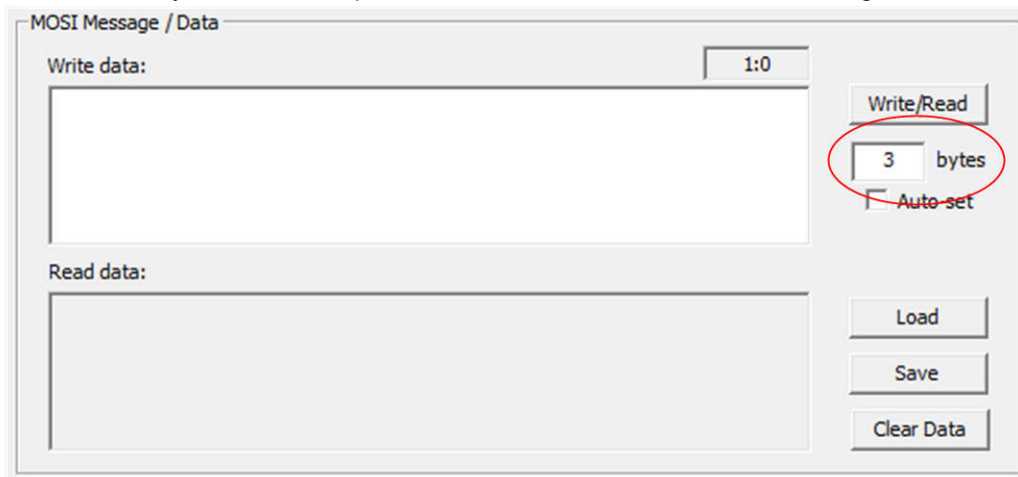
Figure 2-6. Setting Bytes for SPI Communication
