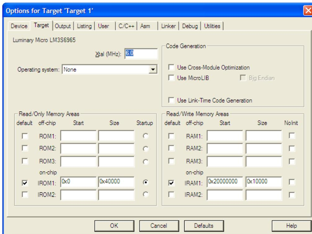
Here you need to set up the Xtal frequency for your specific board. This step is important because the value of the Xtal field is used to calculate flash programming timing later on. Also check the ROM/RAM sizes to make sure that it corresponds to the device you have.
