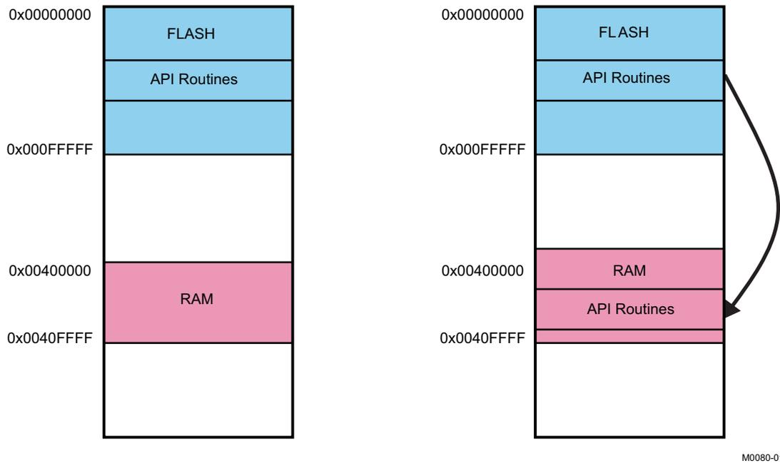
Figure 3. Diagram Showing the API Routines in Flash Memory and Copied to RAM
