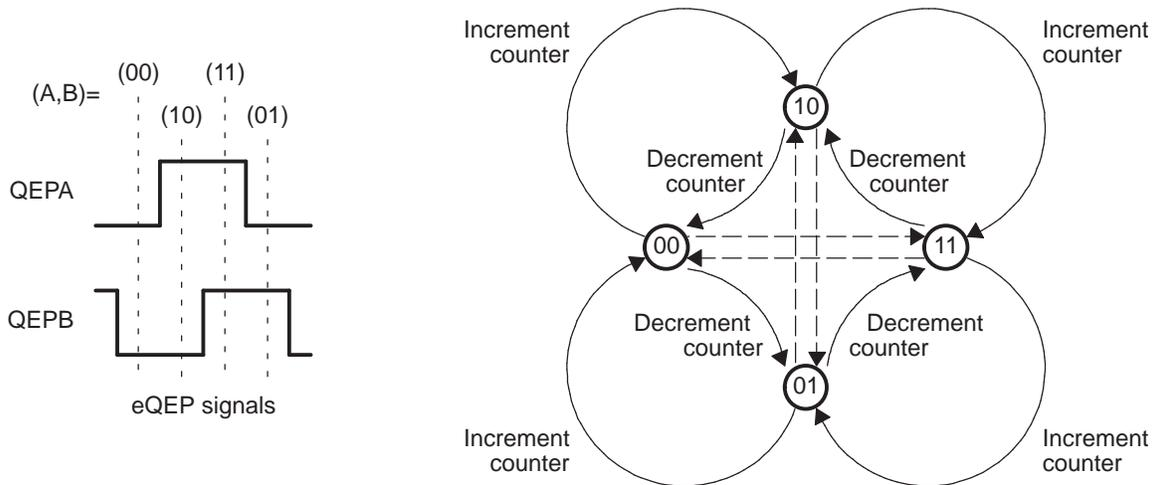
**Figure 3. Quadrature Decoder State Machine**
