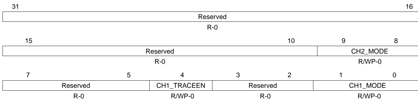
Figure 14-11. CRC Global Control Register 2 (CRC_CTRL2) [offset = 10h]
