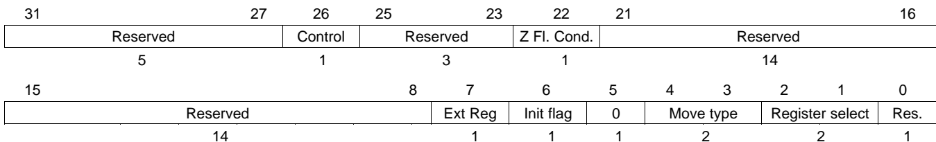
Figure 23-154. MOV32 Control Field (C31:C0)
