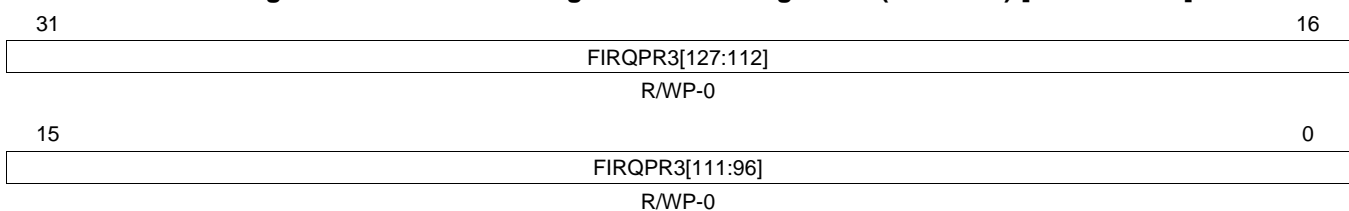
Figure 15-20. FIQ/IRQ Program Control Register 3 (FIRQPR3) [offset = 1Ch]
