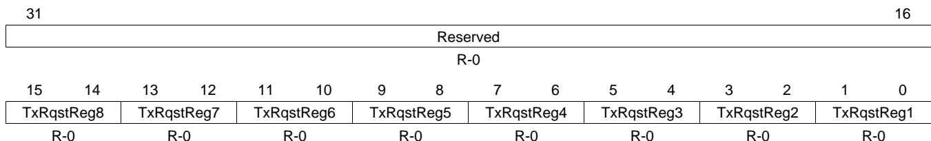
Figure 26-28. Transmission Request X Register (DCAN TXRQ X) [offset = 84h]
