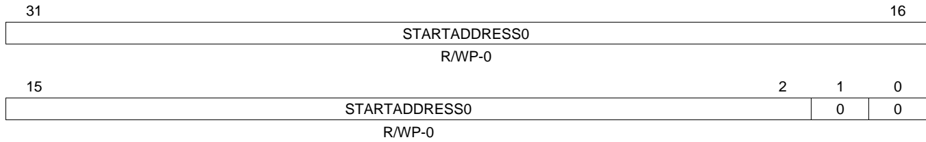
Figure 24-40. Memory Protection Start Address Register 0 (HTU MP0S) [offset = 74h]
