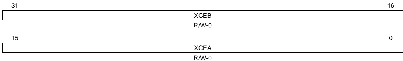
Figure 60. Transmit Channel Enable Registers (XCER)
