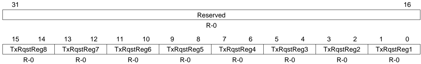
Figure 5-27. Transmission Request X Register (DCAN TXRQ X)
