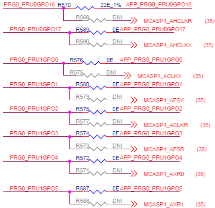
Figure 23. Multiplexed RGMII/McASP1 Signal Selection
