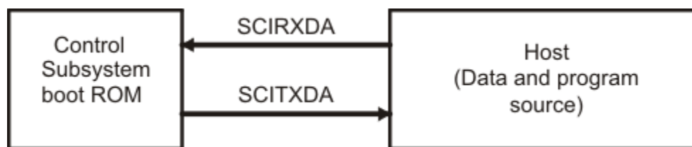
Figure 4-4. Overview of SCI Bootloader Operation
