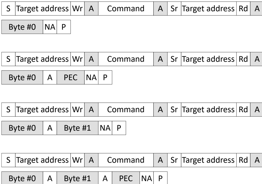
Figure 29-6. Read Byte and Read Word Messages With and Without PEC
