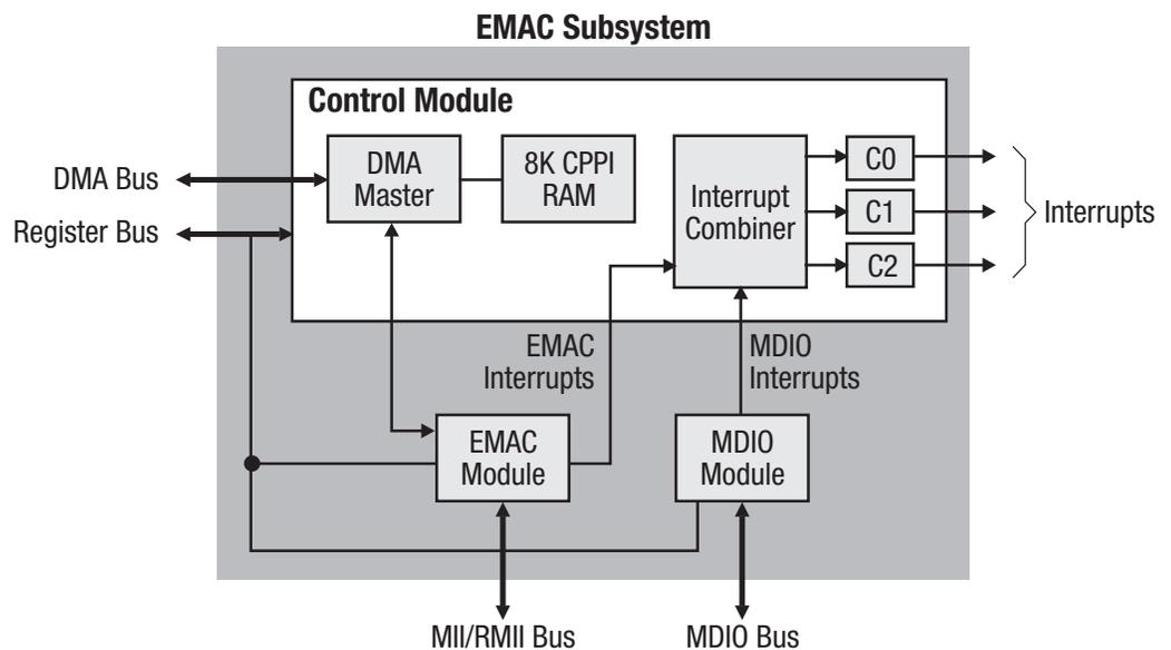
Figure 3. EMAC subsystem.
