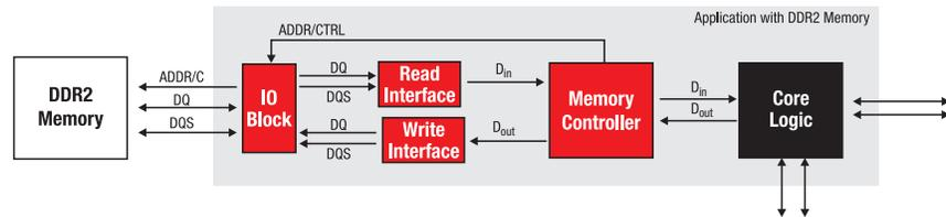
**Figure 4. Simplified DDR2 controller implementation**
