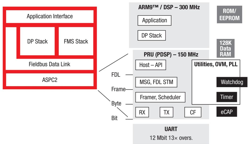
Figure 1. PRU implemented in a PROFIBUS application
