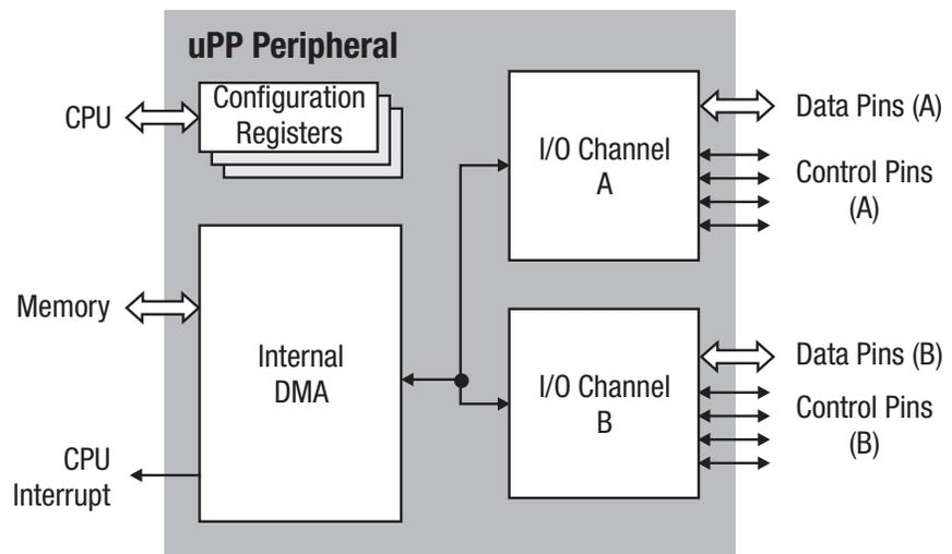
Figure 2. uPP simplified block diagram.
