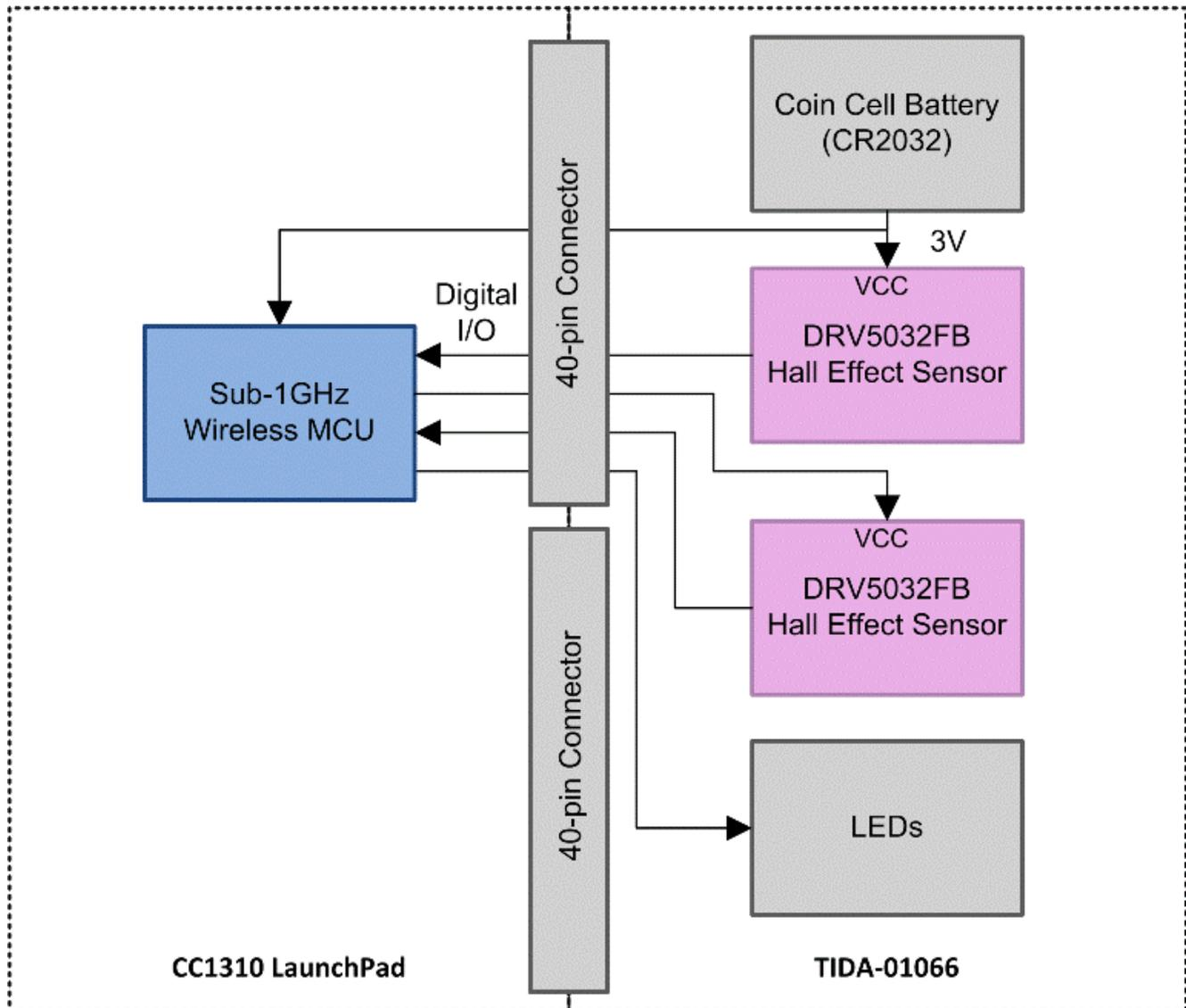
**Figure 2. Block Diagram of TI's Door and Window Sensor Reference Design**
