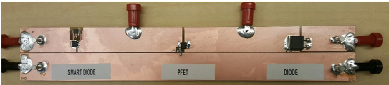
Figure 1. Board Used for Comparison of Thermal
