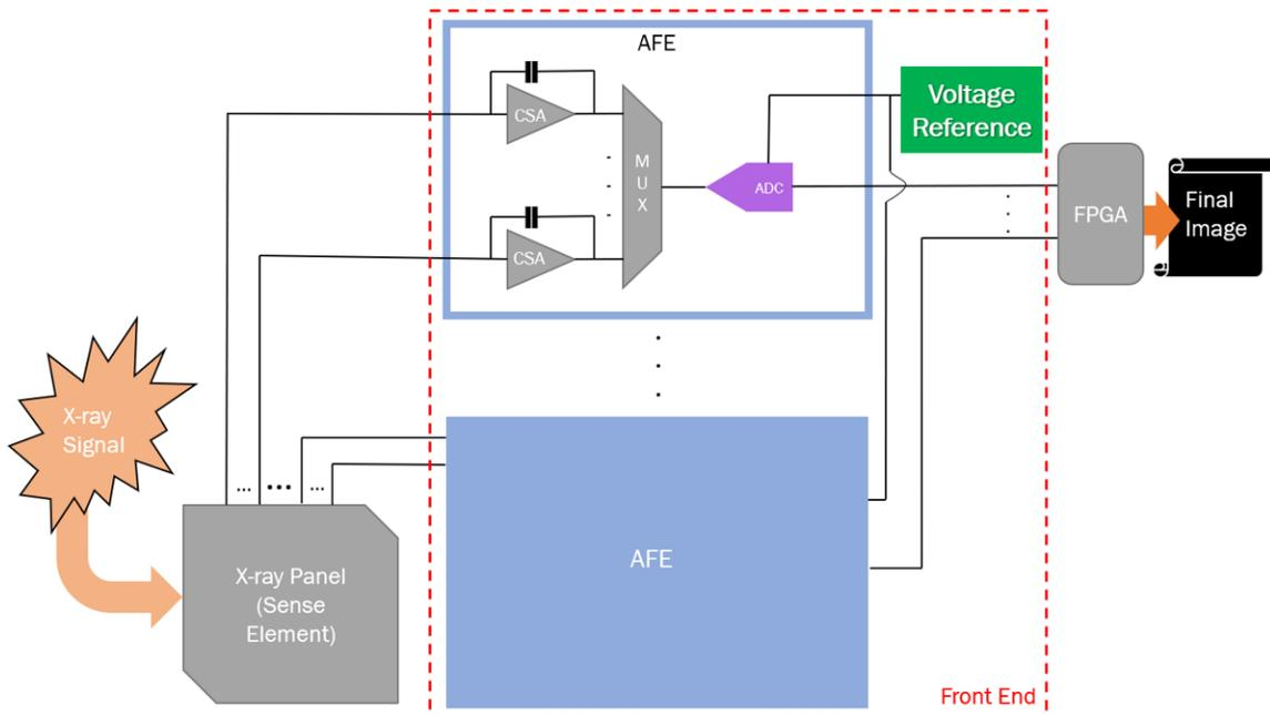
Figure 1. Simplified block diagram of an X-ray system front end
