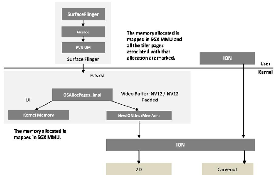
**Figure 5 - Overview of Buffer Management Components in A404 BSP.**
