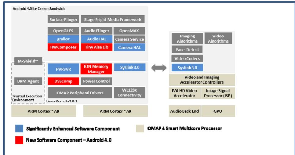
**Figure 1** - Android 4.0 OMAP 4 Board Support Package (A404 BSP) Architecture Overview (Selected Components)
