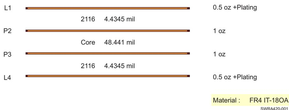
**Figure 1. PCB Stack-Up**
