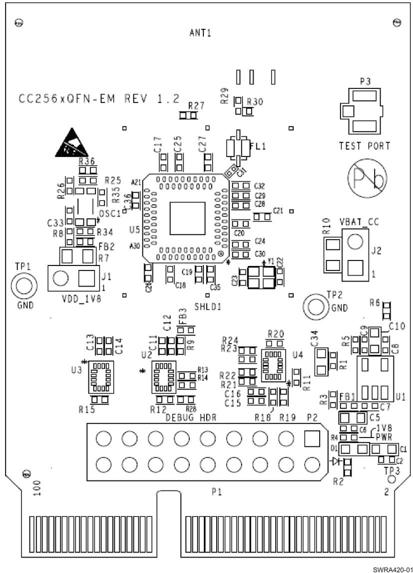
Figure 17. CC256x QFN EM Board – Top Side
