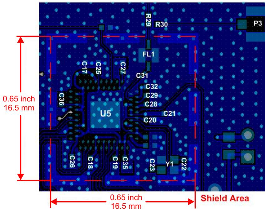
Figure 3. Component Placement
