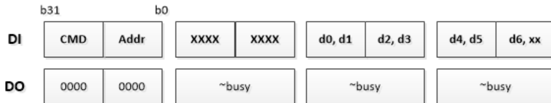
Figure 3-2. 32 Bits, Big Endian, Write Direction
