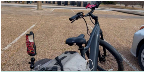
Figure 3. IWRL1432BOOST-BSD EVM Mounted on the eBike
