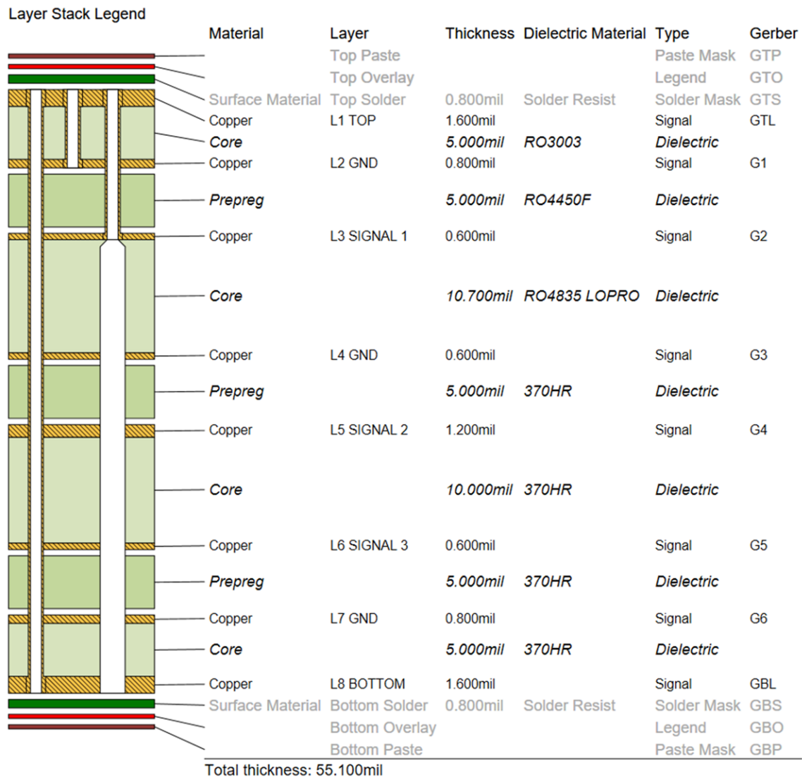
Figure 30. MMWCAS-RF-EVM PCB and Drill Stack-Up Table
