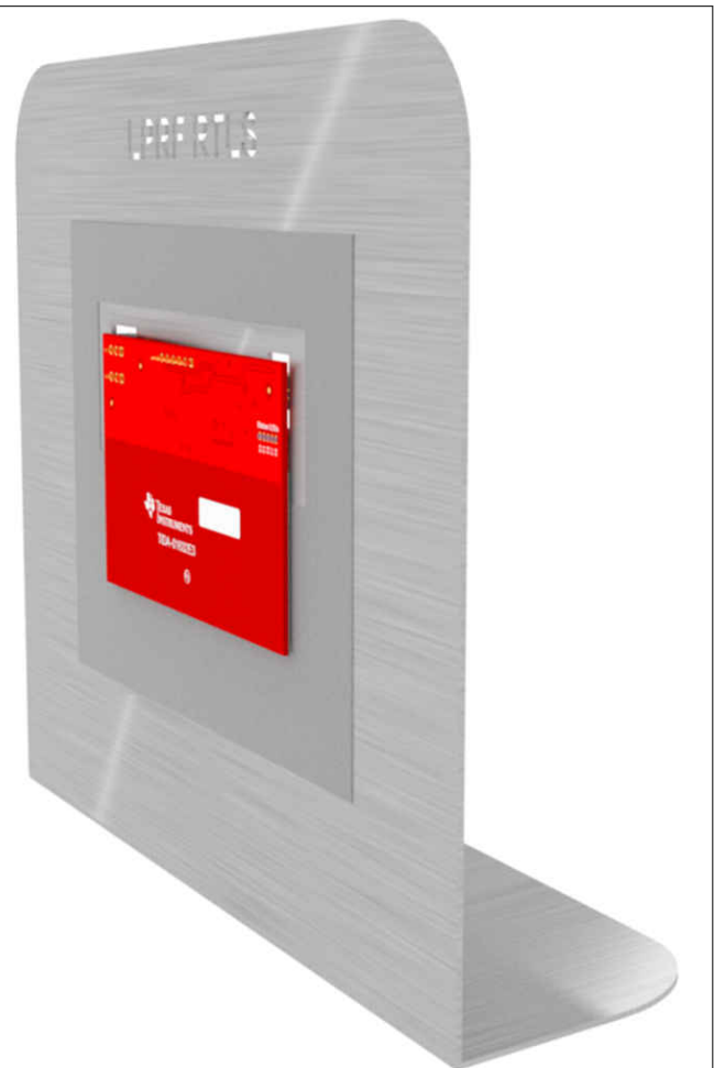
Figure 3-44. PCB + RF Absorbing Material + Tin-Plated Copper Foil + Metal
