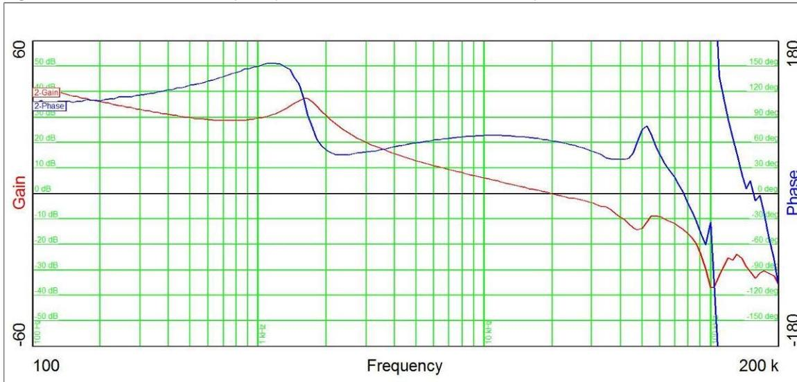
The crossover frequency 20kHz fits exactly to the first calculation by hand, the phase margin is more than 60 degrees. Slope at crossover is close to -1.
