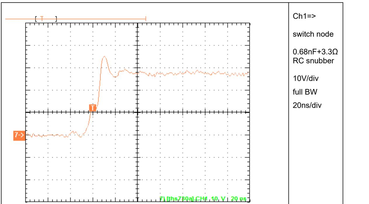
Clamping network 0.68nF / 3.3 Ohm reduces RF content at the switch node, less EMI !
