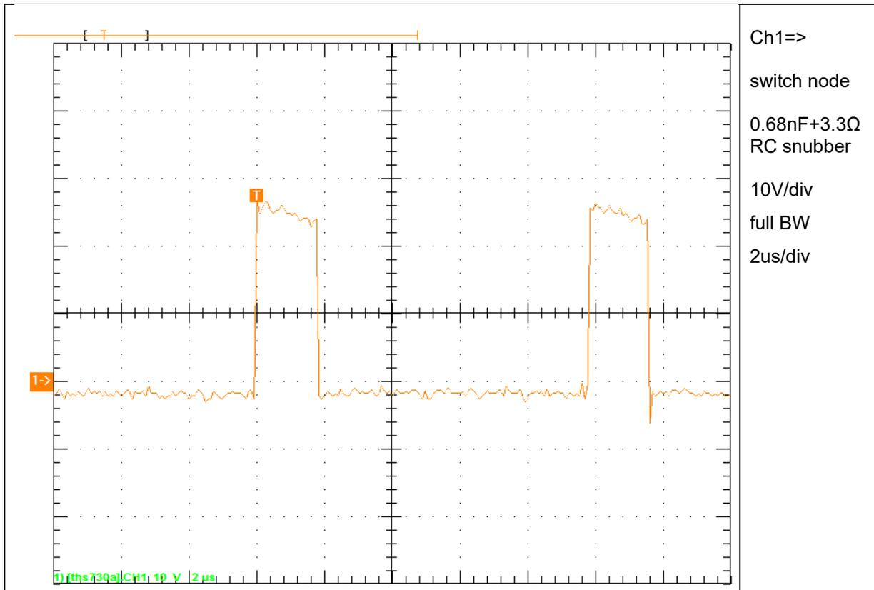
By experience could be said that a drop in efficiency from 0.2% to 0.5% is typically caused by adding the RC snubber circuit. For a middle power design like PMP30600 geometry 1206 or 1210 might fit, but for high power designs be aware of losses up to 500mW:
