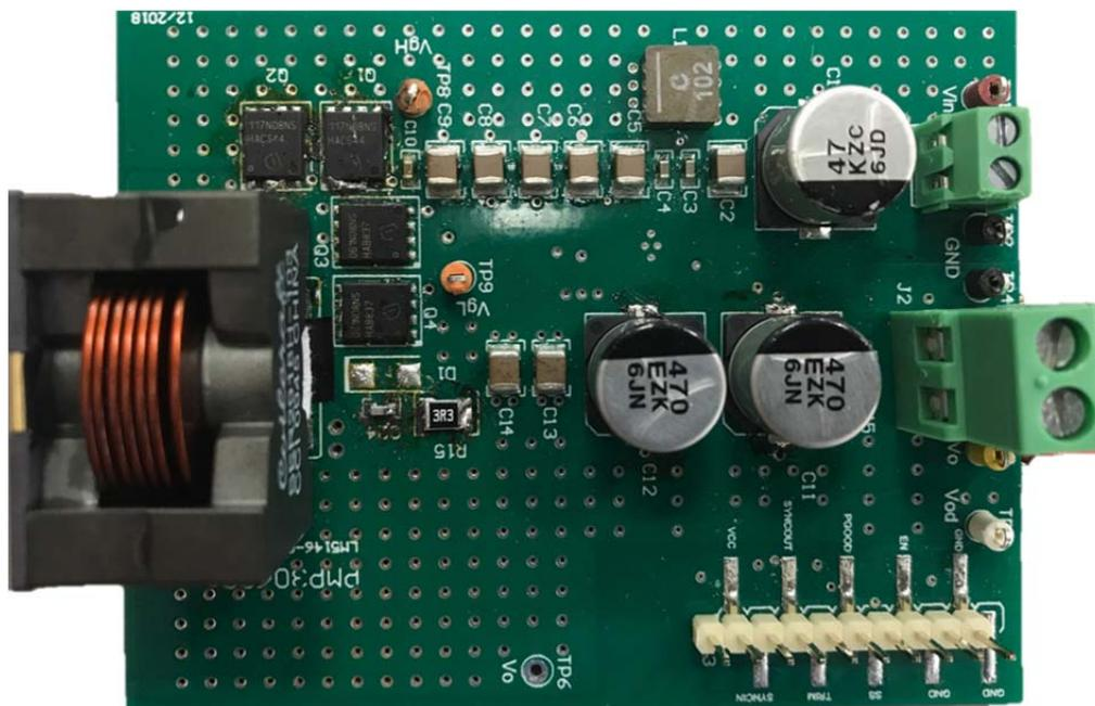
Filter inductor and RC snubber have been placed externally
