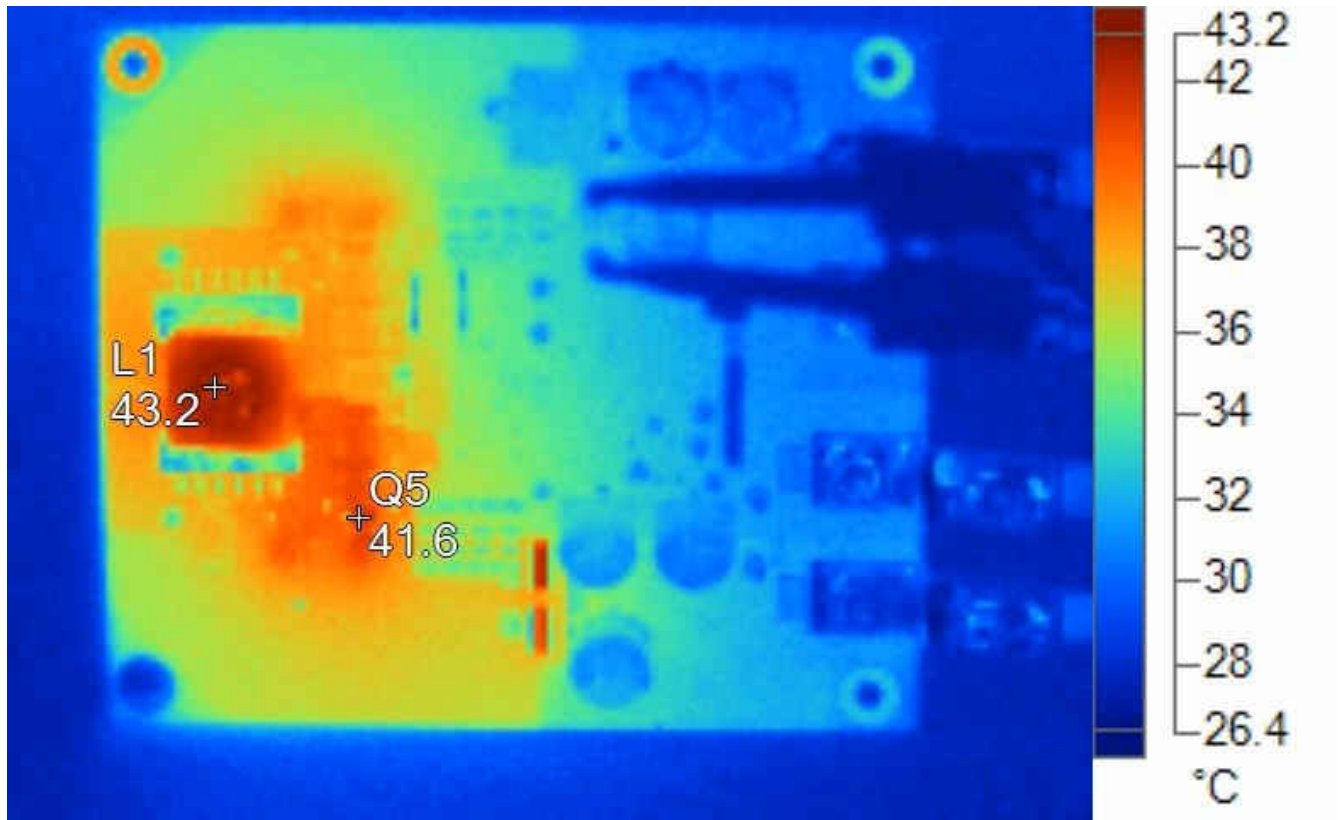
Figure 2-22. 12.0 V IN , 30 A OUT , Continuous Operation, Transition Mode at ½ F SW
