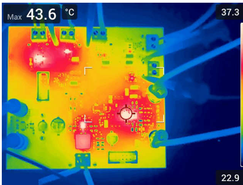
Figure 2-7. Thermal Image, 12-V Input, Full Load Output With 0.75-V VDD_CORE With 5.7-A Load
