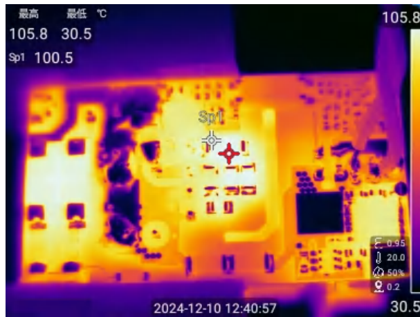
Figure 2-17. 90VAC, Dual Port, 45W (15V, 3A) +20W (9V, 2.25A), Full Load, PCB Bottom Side
