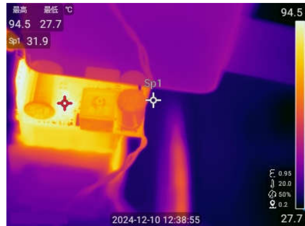
Figure 2-18. 90VAC, Dual Port, 45W (15V, 3A) +20W (9V, 2.25A), Full Load, DCDC Board
