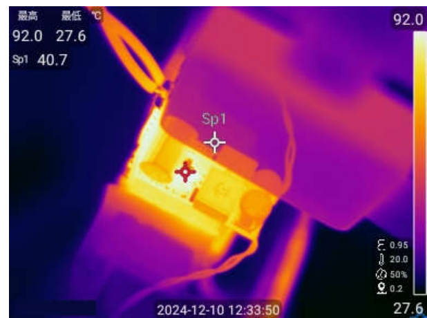
Figure 2-20. 264VAC, Dual Port, 45W (15V, 3A) +20W (9V,2.25A), Full Load, DCDC Board
