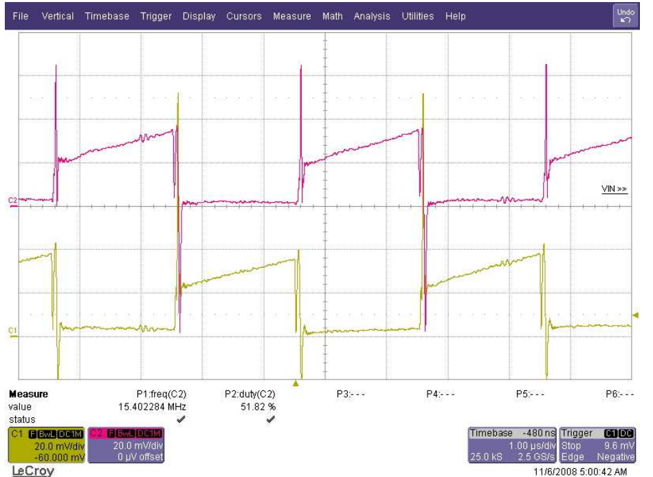
Current Sharing 4 (Vin=9V Iout=5A): CsenseQ1 (C1), Vsense Q2 (C2)
