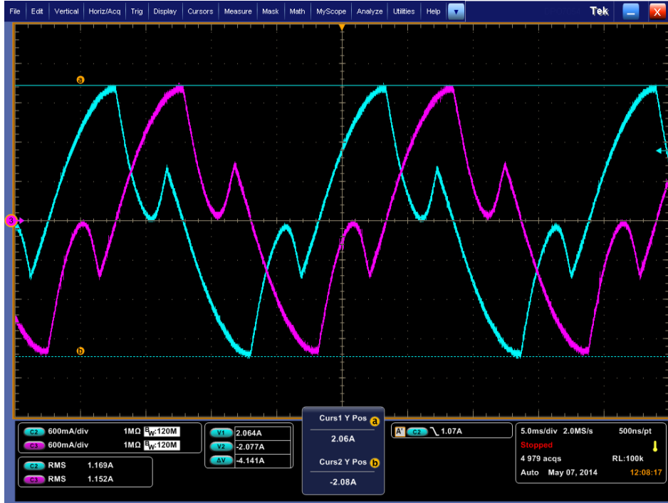
Fig. 33 256 \mu Step / Auto Mixed Decay, t_{off}=36\mu s
