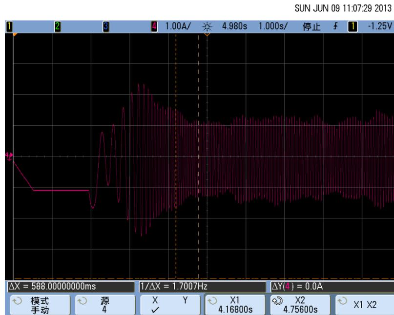
**Figure 8. Start-up with Load**
