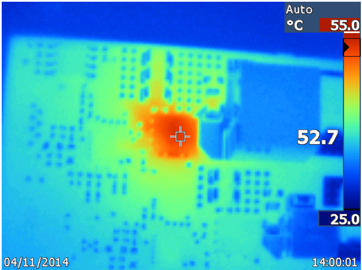
Figure 26. VIN = 5V, VOUT = 1.0V, IOU = 24A Thermal Image
