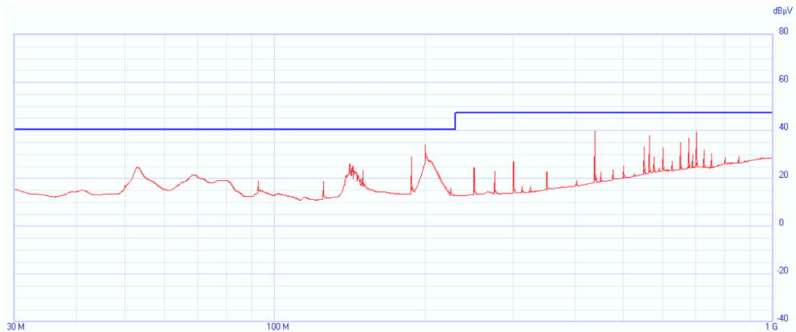
Figure 21. Media_Converter_100Base-T to 100Base-FX_ClassB
