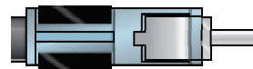
The SC connector for fiber features a molded body and a push-pull locking system.
