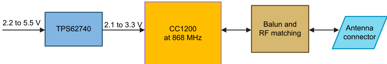
Figure 3. Block Diagram of CC1200 wM-Bus RF Subsystem at 868 MHz
