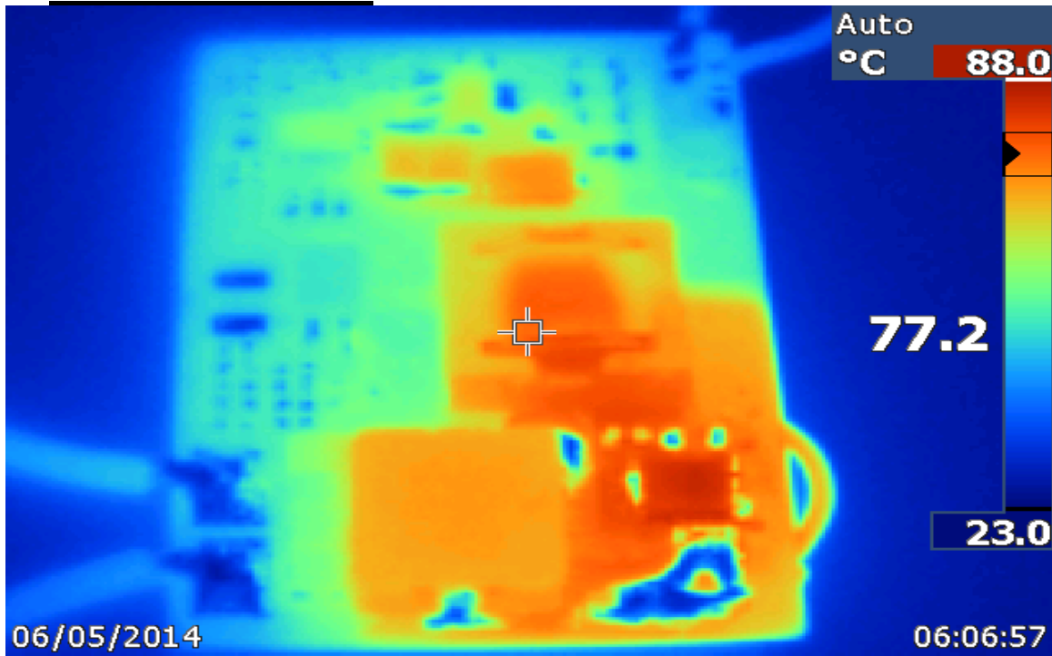
Top side, 40Vdc and 6A load, T_a=25^\circ
