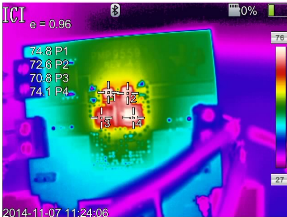
10Vin, 7V/6A, 5V/6A, 300kHz, Tamb=25C, natural convection. P1: 7V-FET; P2:5V-FET; P3:7V-IND;P4:5V-IND.
