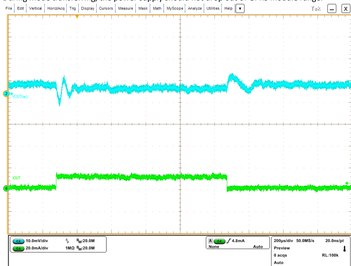
Figure 6 Transient Response during Transfer between SLEEP and IDLE Mode
