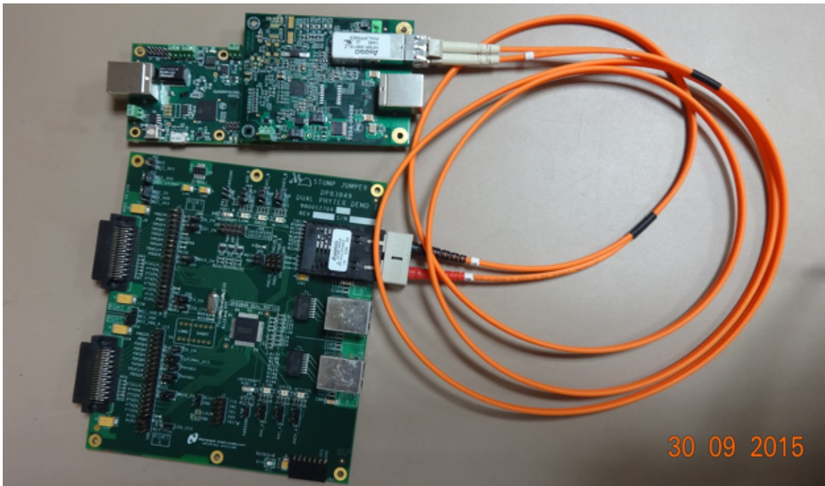
Figure 15. FO Board Connection for Testing
