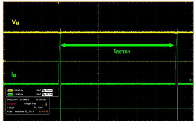
Figure 4. OCL  $t_{RETRY}$  interval
