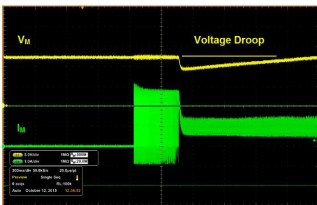
**Figure 1.**  $V_M$  Droop Without Current Limiting
