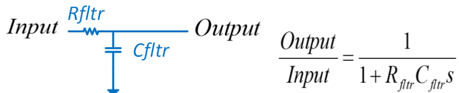
Figure 6. RC Filter
