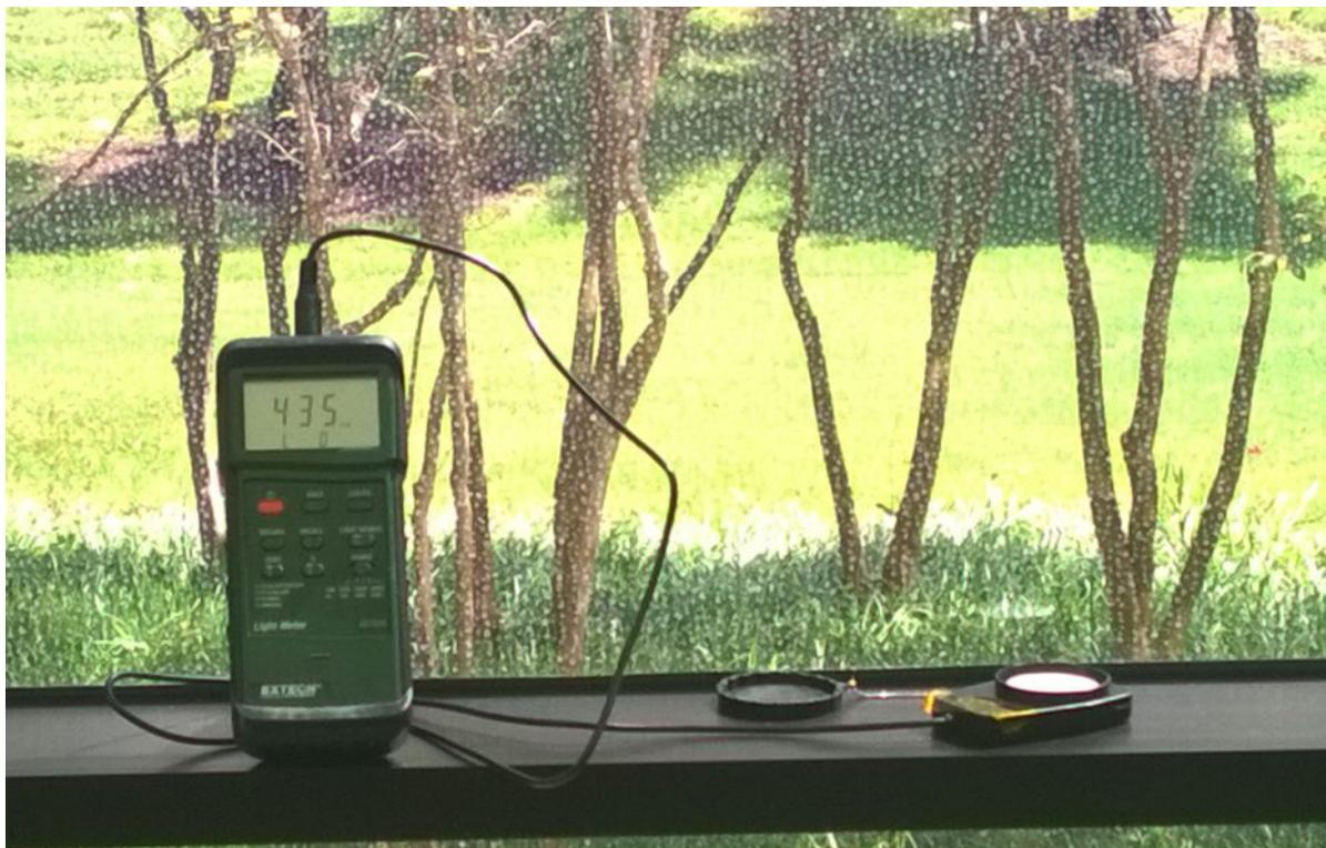
**Figure 18. Light Meter Measuring Light Level in a Sunny Window**
