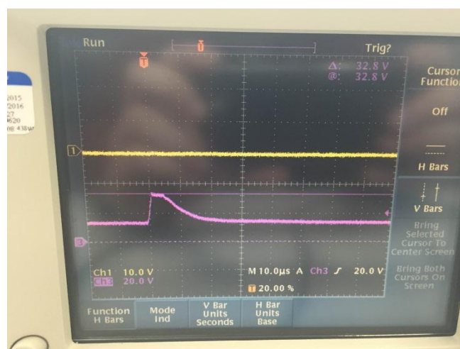
Figure 41: Input pulse is clamped to 32.8V by TVS diodes
