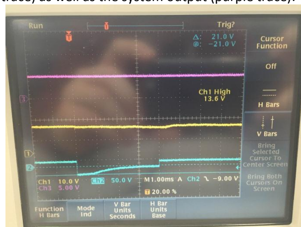
Figure 36: TVS circuit clamps the negative voltage to -21V
