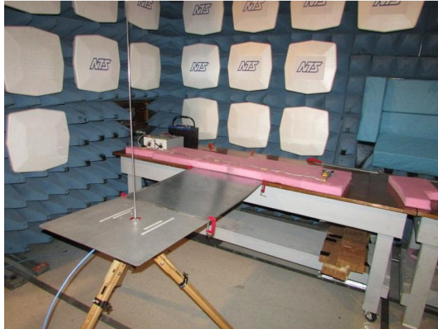
Figure 55: Radiated emissions setup with monopole antenna
